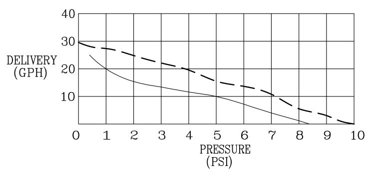
MINIMUM PRESSURE VS. DELIVERY CURVE AT NOMINAL VOLTAGE. ZERO HEAD ON FUEL INLET AND OUTLET.
